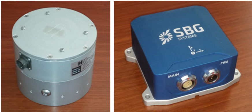
Fig. 5.10 The Hyperion IFS-5000 microbarometer sensor (left) and the SBG inertial measurement unit (right)
